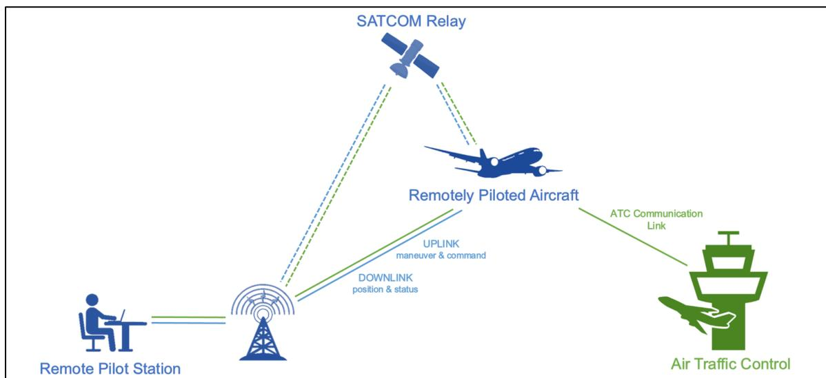
Figure 1. Example of C2 and ATC communication link architecture.
