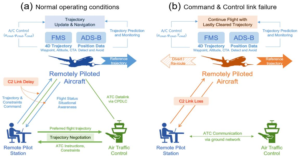
Figure 3. Schematics of Trajectory Based Operation with C2 link architecture. (a) C2 link delay affects both uplink (updating trajectory and constraints) & downlink (flight status). While ATC CPDLC message and the aircraft control does not directly influenced. (b) When C2 link fails, RPA continue flight with the lastly cleared trajectory till C2 link recovery.
