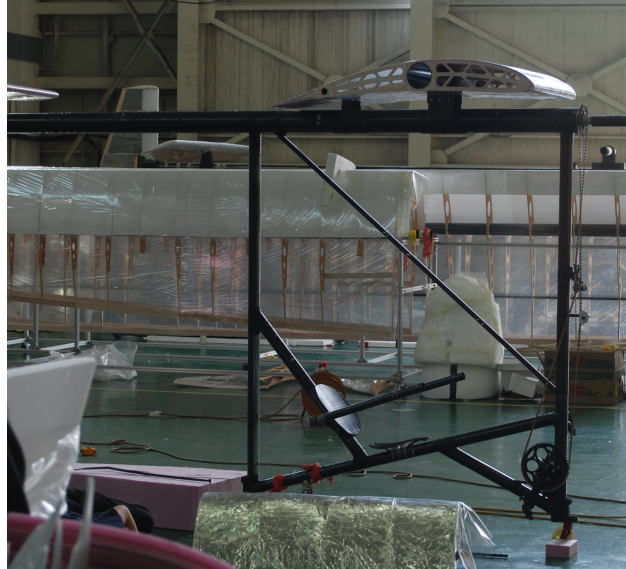
Fig. 1 Front part of the fuselage of the 2015 HPA with almost no overhang.
