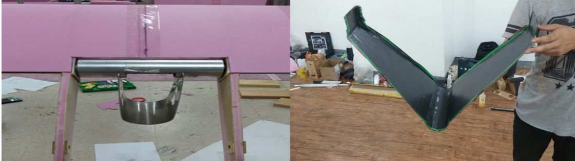
Fig. 11 Bracket for tails (Left: aluminum construction for 2014 HPA, Right: CFRP construction for 2015 HPA)
