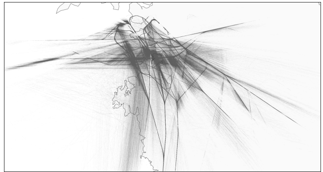
Fig. 7. Recorded ADS-B Trajectories
