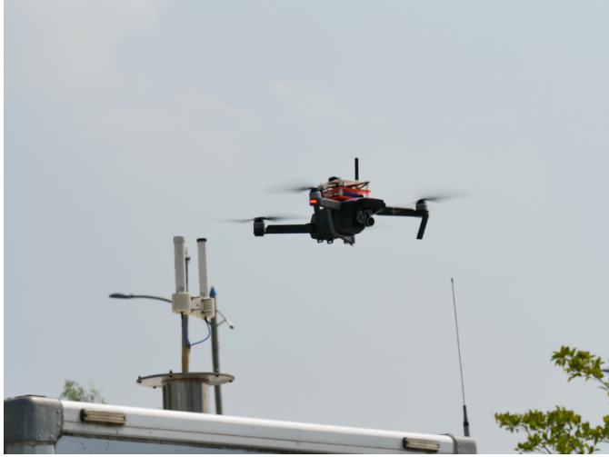
Fig. 3: TR-1A ADS-B transceiver installed on a DJI Mavic Pro drone
